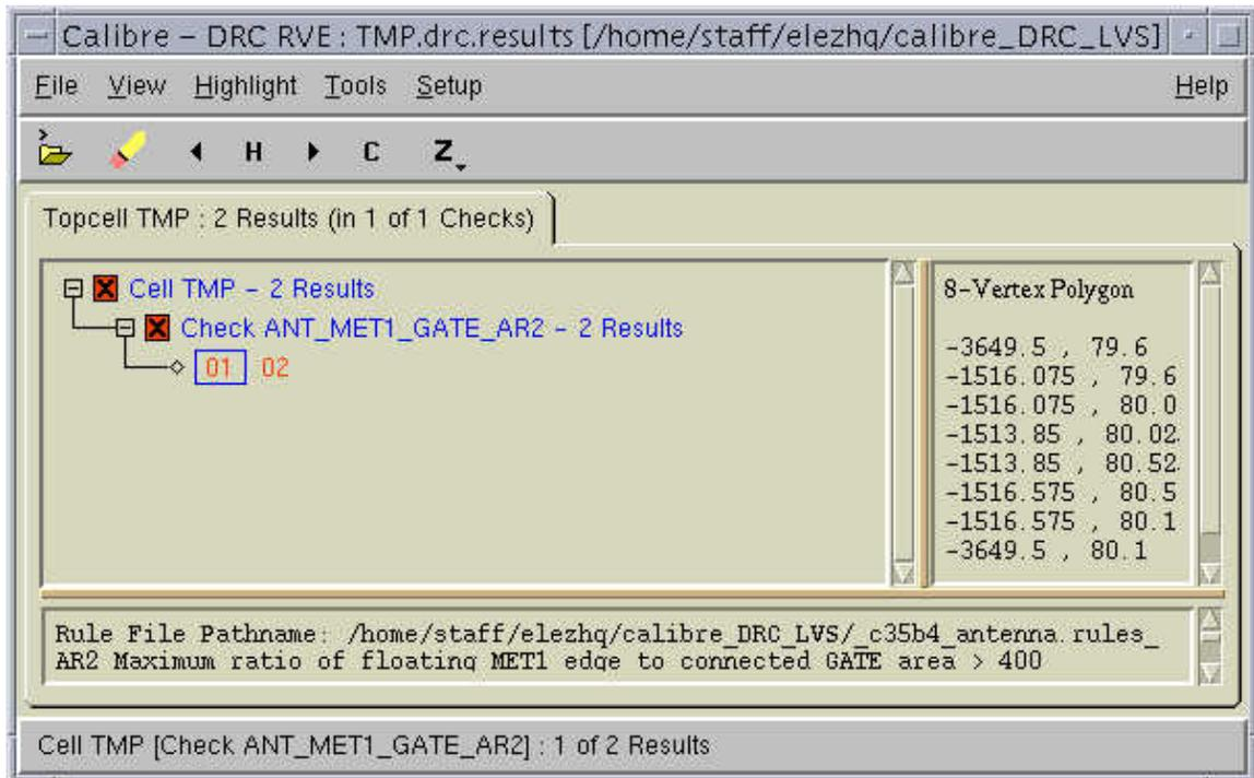
Fig 7. Highlight error in Calibre – DRC RVE window.
