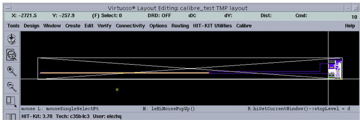
Fig 8. Errors highlighted in the layout window.
